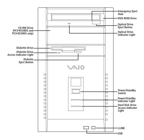
For your convenience, your computer includes USB and i.LINK connectors on both the front and back panels, allowing you to connect to either set of connectors. The i.LINK connector on the front of your system is a 4-pin connector.
